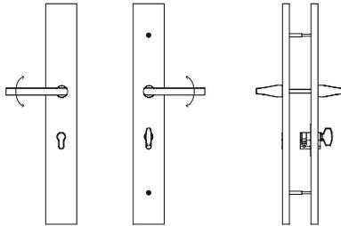
**Non-Keyed with Cylinder Plugs, Fixed Handle Outside, Operating Handle Inside** (for Semi-Active Door)
